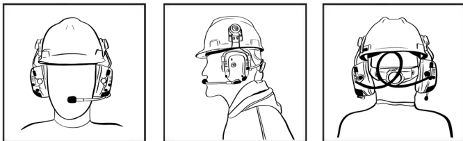
FIGURE 5 - Helmet Mount Fitting Instructions
