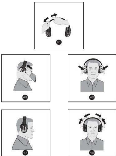
FIGURE 4 - Headband Mount Fitting Instructions
