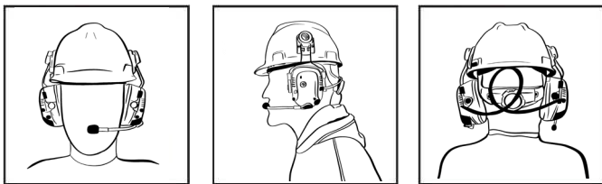
FIGURE 5 - Helmet Mount Fitting Instructions
