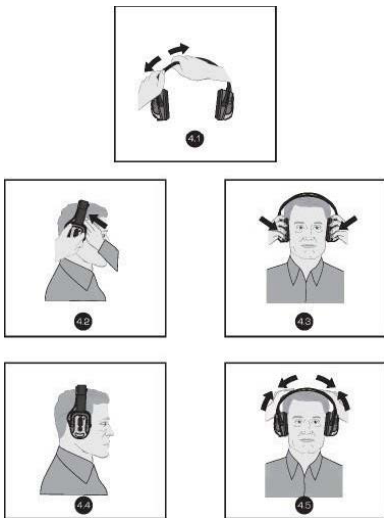
FIGURE 4 - Headband Mount Fitting Instructions
